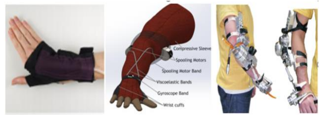
Fig. 3. Classification of orthoses according to the type of suppression: a) passive, b) semi-active, c) active
