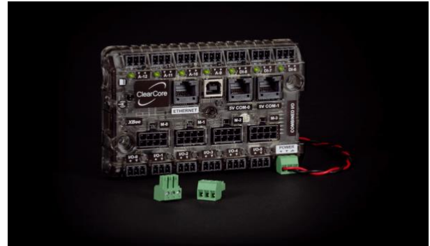
Fig. 3. ClearCore - Industrial motion and I/O controller [3]
